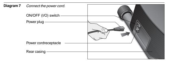
11. **Connect the power cord.** Diagram 7. Insert the power plug's connector into the receptacle at the rear of the base assembly.
